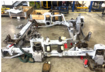
One of the Brill 22E bogie frames being reassembled after significant maintenance. Photo: Paul Mong
